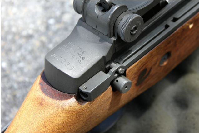
Figure 4.56 Close-up of the receiver markings of the H&R M14. Note the selector switch knob on the right side of the receiver. Semiautomatic copies of the M14 generally do not have the notch cut in the stock for the selector, although surplus stocks in circulation may or may not be cut for the selector. (Image from author's collection.)
